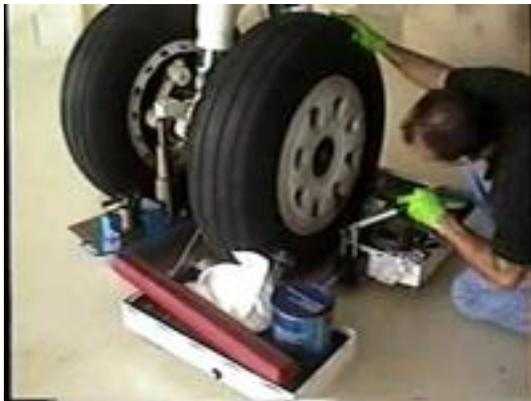
Visually align the wheel hub to the aircraft axle, make fine-tuning adjustments by pumping or bleeding hydraulic pressure on the wheel dolly. Rotate the wheel as needed to align with brake keys.
