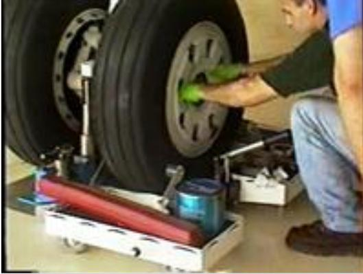
Verify proper unpacking, correct wheel guide slot determination, and opening of wheel dolly.
